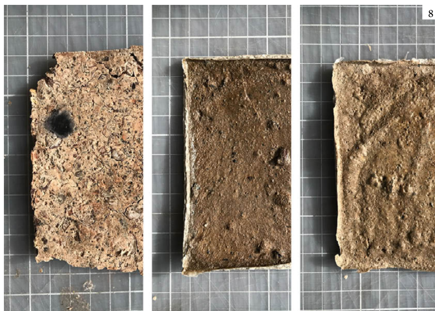
Figure 8 Material experimentation with cashew nutshell and ash, 2023.
