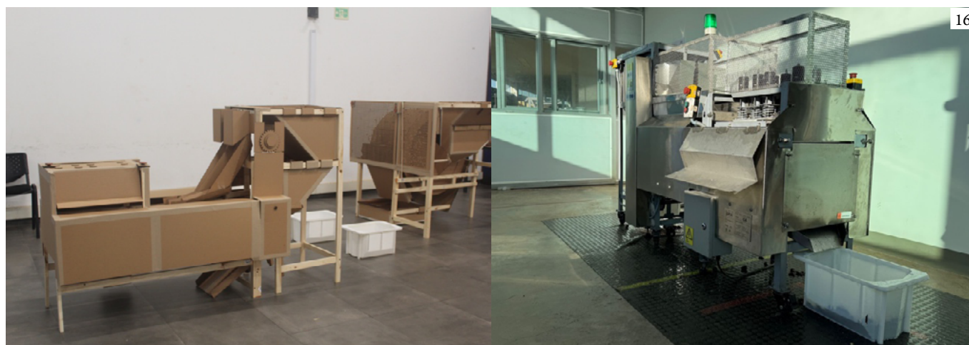
Figure 16 Low resolution prototypes and final machinery development for cashew nutshell opening and separation, 2025.
